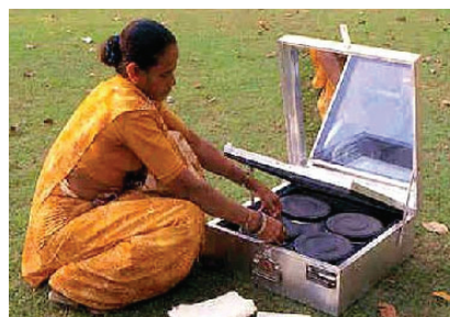
Fig. 12.4 Box type solar cookers
